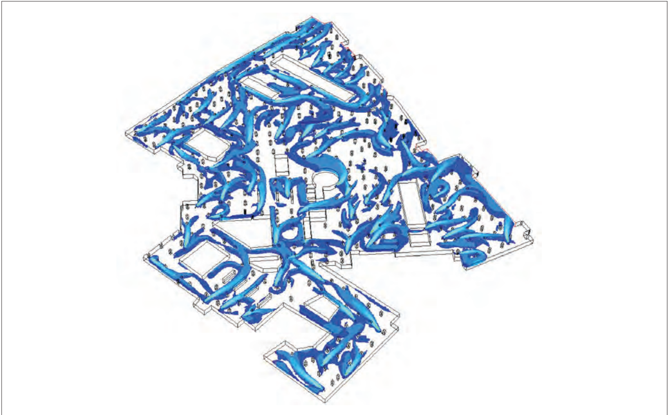
Iso-plane tracing of 0.5m/s velocity region for normal operation (Pollution control)
