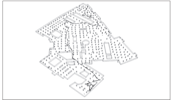
Smoke path tracing in a car park
