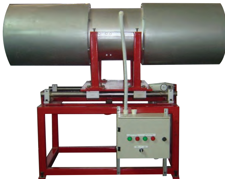
Special Test Rig constructed in accordance with ANSI/AMCA 250-05
